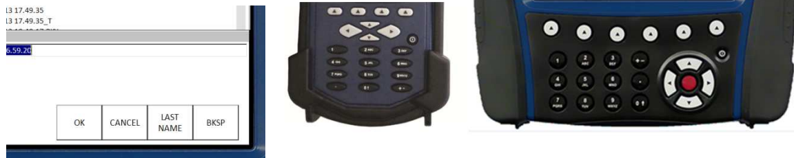
Figure 10: All Modules – Storing of the last entered filename; i.e. the possibility to recall -within a firmware Module- via the function key „LAST NAME“ (left) / comparison of VT-80/VP-80 key pad with function keys, alpha numeric keys and Cursor cross with Fire Key for quick navigation (right)
