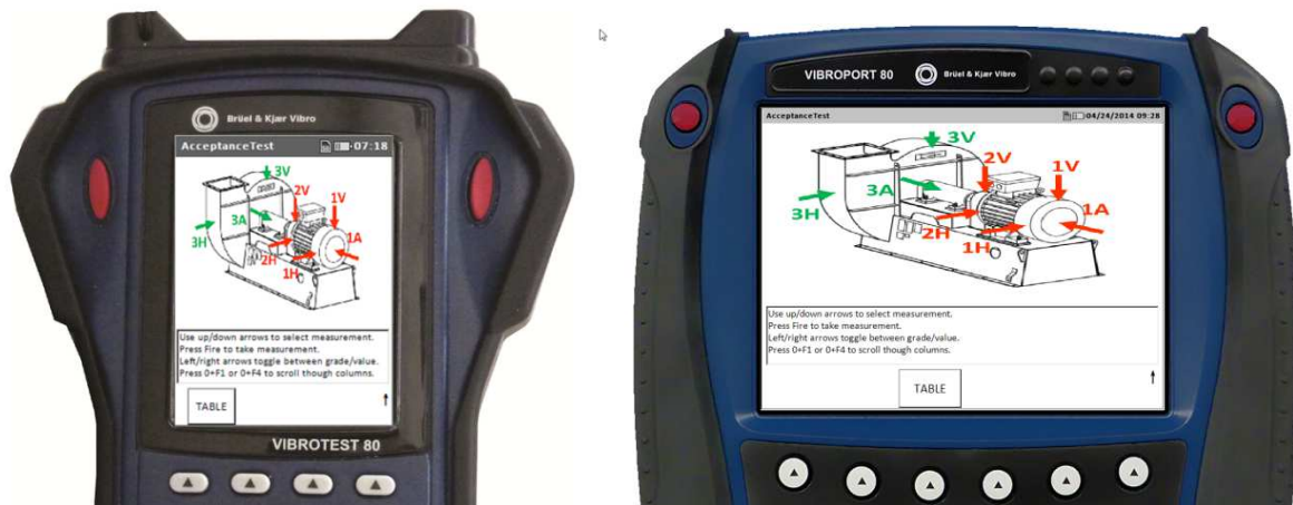
Figure 9: Module 11 Acceptance – Displays of customized integrated machine picture *.bmp for better orientation (VT-80 left / VP-80 right)
