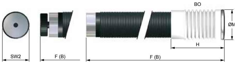
Material: PTFE / Stop cap: stainless steel Ordering information: WS-M 0,25 - 1BO
